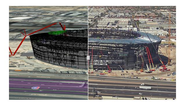
EarthCam, a provider of webcam technology and services, has introduced EarthCam 4D, empowering virtual design and construction (VDC) teams to overlay and sync live imagery with their digital twins. An intuitive time-line allows users to scroll backward and forward in time to view live imagery in relation to their 4D models.
