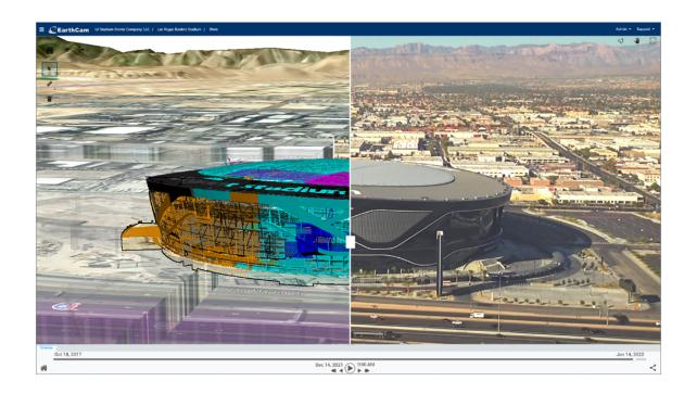
EarthCam has introduced EarthCam 4D, designed to empower virtual design and construction (VDC) teams to overlay and synch live imagery with their digital twins.
