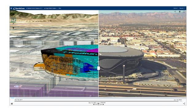
A new tool has been created by Earthcam that is said to make it easier for those in construction to view the progress of projects compared to their initial design plans, and make the digital twin process simpler.
