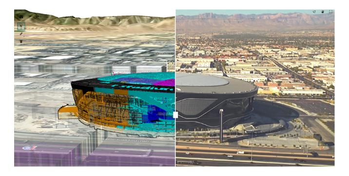
Built on the Bentley iTwin platform, EarthCam 4D augments Bentley Systems' SYNCHRO 4D models with high-resolution photos from multiple cameras throughout the jobsite.
